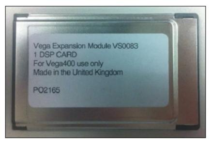
Insert the DSP card into the top slot (label face down).NOTE: Make sure to push the card all the way into the slot until the push notch comes all the way out.
